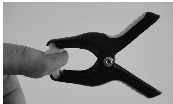
Figure 1 Mechanical spring clamp. Generic, inexpensive wood-working spring-clamp.
