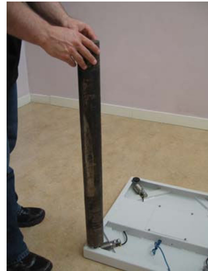
Figure 3 Placement of weight during calibration of force platform.
