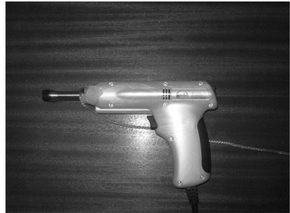
**Fig. 1** Impulse adjusting instrument set on the second force setting (200 N). The stylus base was connected by a ground wire to the screened floor to decrease interference on sEMG
